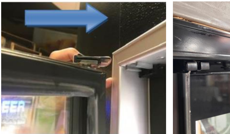
Figure 4.1 Insert Door Hinge Pin to Frame Socket
