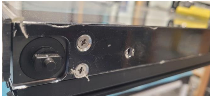
Figure 2.1 Hydraulic hinge tab at “Zero-degree” position
