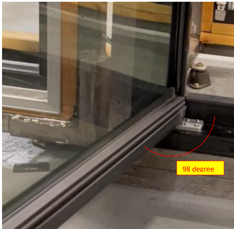
Figure 3.1 Seating door into hydraulic hinge adapter plate.
