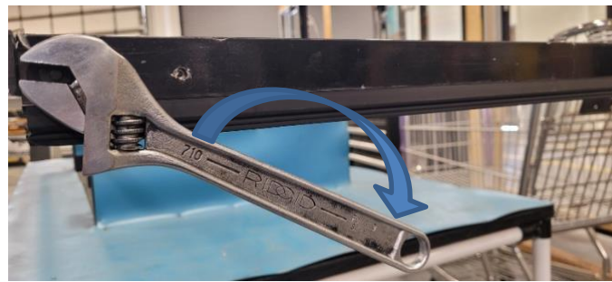
Figure 2.2 Rotating clockwise using at least a 10” crescent wrench.
