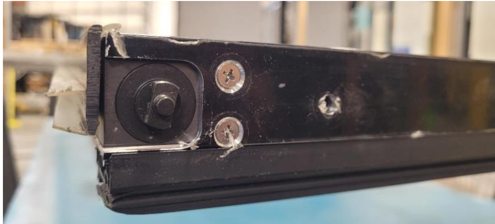
Figure 2.4 Detent position (approximately at 98 degrees)
