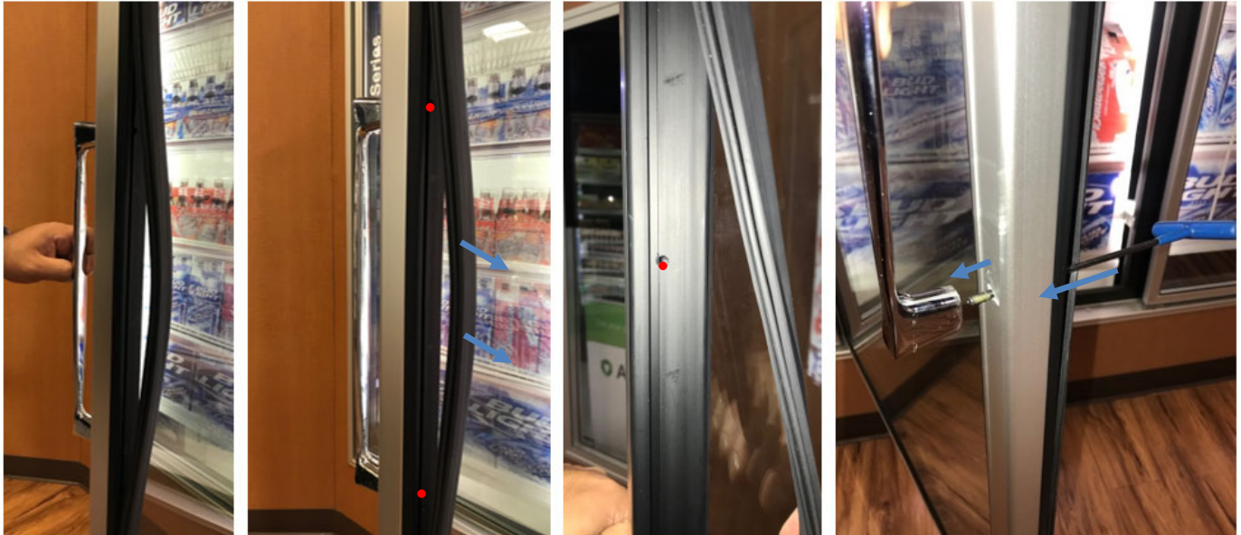
Figure H.1 – Locating handle screws
