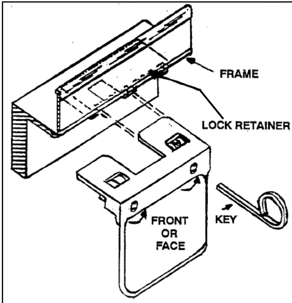
3. Insert the key into the POM Lock square key hole, then turn the key counter-clockwise to lock.
