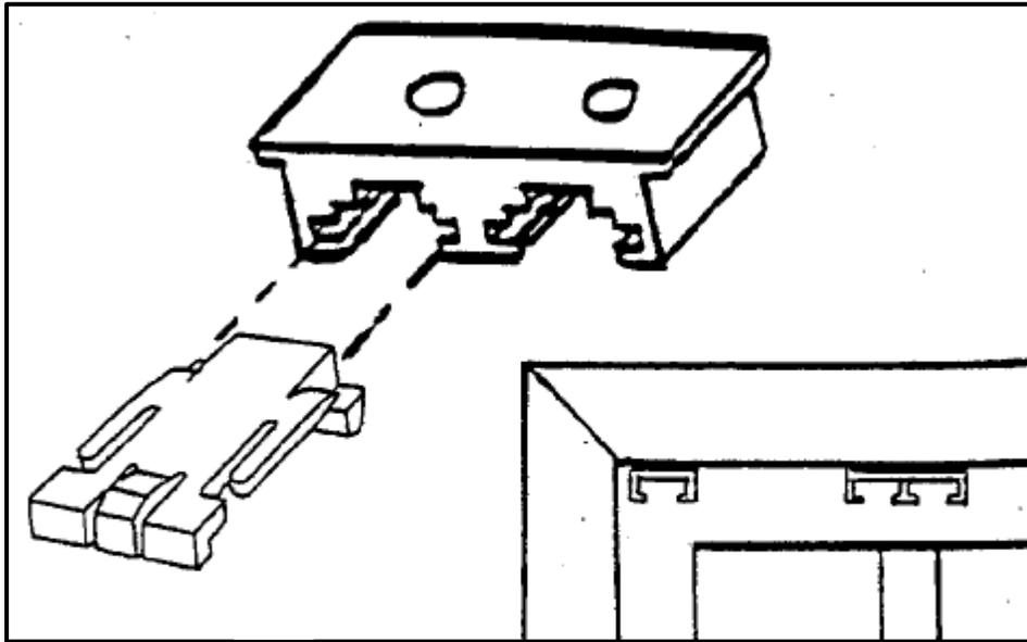
2. The POM Lock inserts into the hinge pin access plate.
