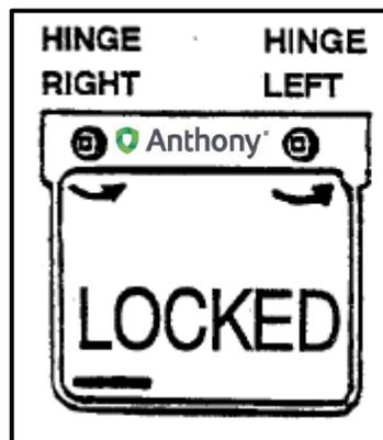
10. The POM Lock always installs in the frame, over the top of the handle rail side of the door.
