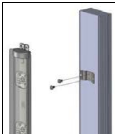
Mounting Clip Alignment
