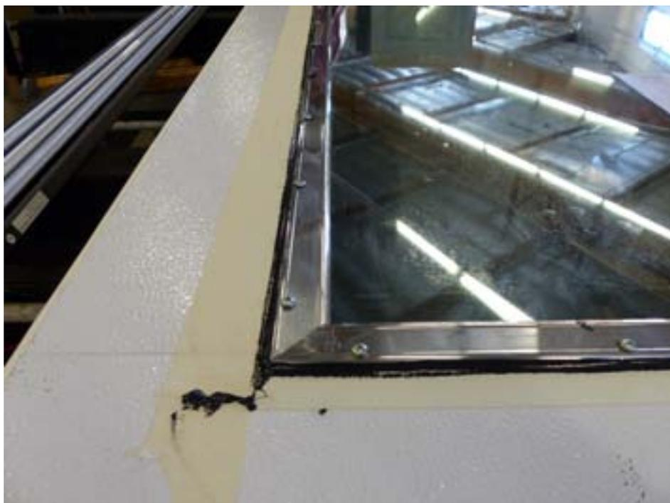
8. Before placing the rear frame in position, drill  $3/16$ " diameter holes in the extrusion as shown. Apply silicone Dow Corning 995 around the entire perimeter of the back frame to assure an air tight seal between the frame and wood and frame and glass unit.
