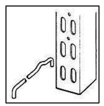
5. After installing the shelves, adjust the rear post leveling bolts to level. The Four-Post Shelving System is now ready for merchandising.
